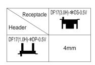
Note: The stacking height doesn't include the solder paste thickness.
